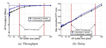
Fig. 8. Impact of statistical multiplexing. There are 1/10 downloads and no uploads. Wired RTT  $200 \mathrm{ms}$ .
